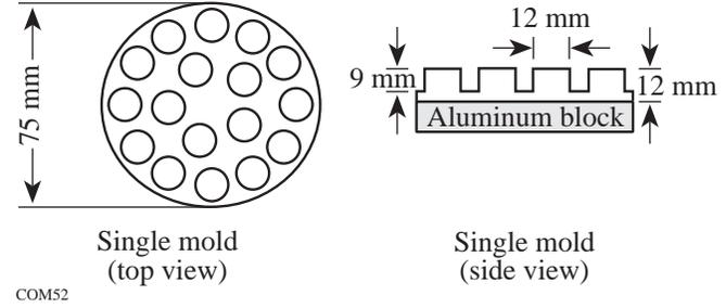
Figure 73.57 Setup for molded pellet array polisher.
