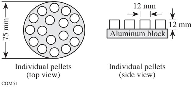
Figure 73.56 Setup for pellet array polisher manufactured from single pellets.
