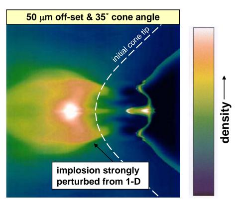
Even with a substantial stand-off of the cone tip from the capsule center a damaging axial jet is directed into the cone tip
