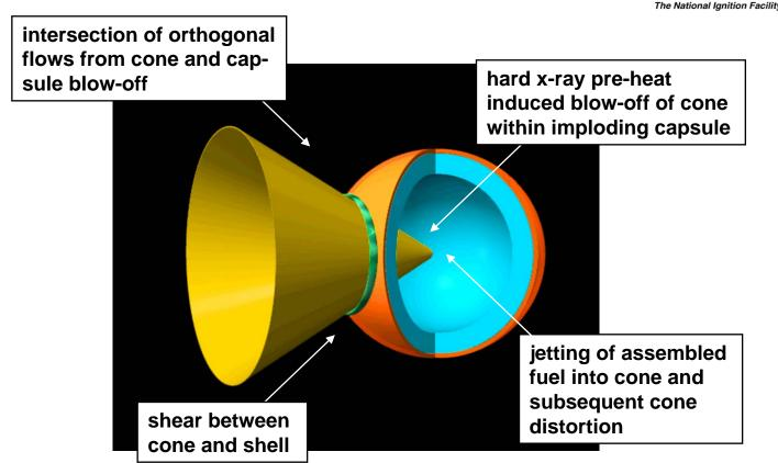
FI targets afford a large design space of parameters (cone thickness, angle, off-set, etc.) which must be scanned for an optimal design
