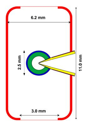
hohlraum geometry with cone is inherently 3-D
