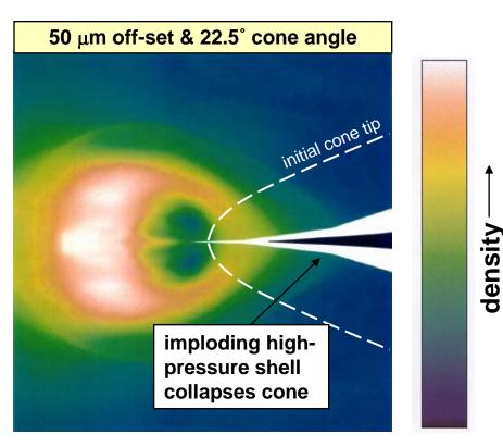
Collapsing of the cone for small angles remains a design challenge — is there an optimal intermediate cone angle?
