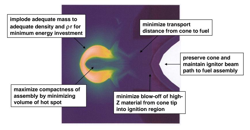
The NIF FI implosion goal is  $\rho \sim 300$  g/cm<sup>3</sup> and  $\rho r \sim 2$  g/cm<sup>2</sup> using 0.6 MJ of compression laser energy
